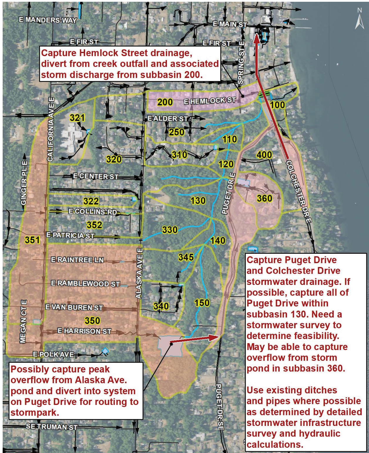
Figure 5: Potential stormwater diversion for: Puget Drive & E. Colchester (4.2.2), Hemlock Street (4.2.3) and Alaska Avenue Regional Detention (4.2.4)
